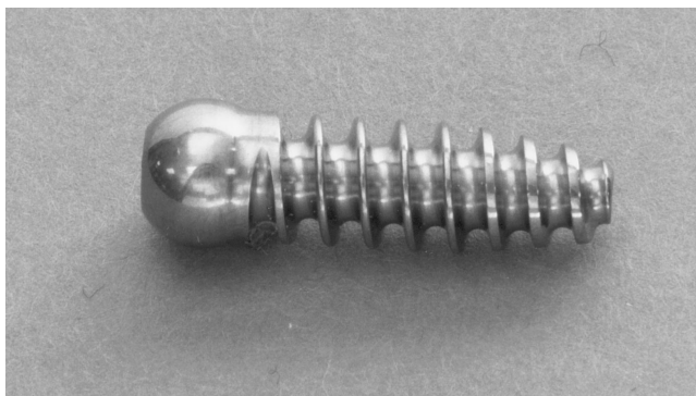
Figure 1. Round-headed, soft-threaded, cannulated, interference screw.
